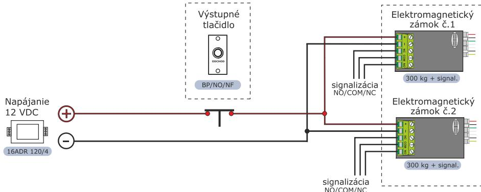
**Príklad č.2:** Prístupový systém + výstupné tlačidlo
